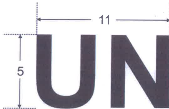
Figure 5 – “UN” inscription on the sides of blue helmet, on ARIAL white font (measurements in centimeters)
